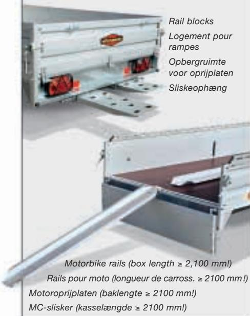
Motorbike rails (box length  $\geq$  2,100 mm!)
