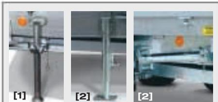
Sliding rail supports [1], or swivel and rotatable, telescopic crank supports [2]
